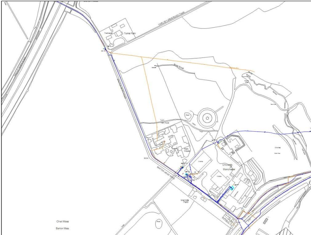
Additionally, there is a pole mounted transformer to the west and directly opposite Tunnell Farm. The orange cable line with runs east on diagram below is out of commission and also does not show on online mapping systems.
